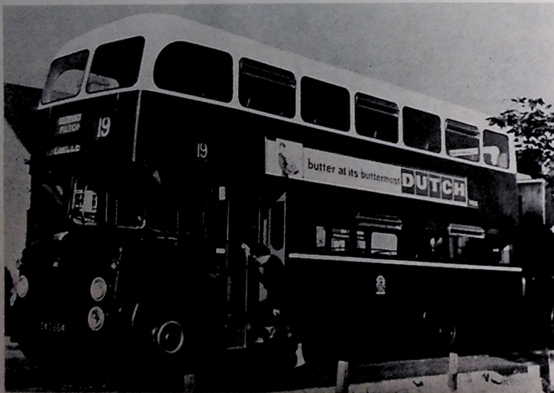
In an attempt to reduce painting time and costs, various simplified liveries have been tried, as on this 30ft. long double-decker. (Block by courtesy E.C.T.)
