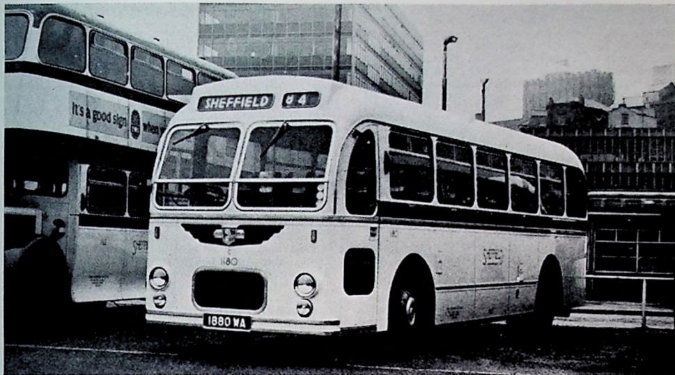
An unusual combination—Leyland Leopard chassis with Eastern Coachworks body (see SHEFFIELD TRANSPORT below). (Block by courtesy of "Modern Transport")
