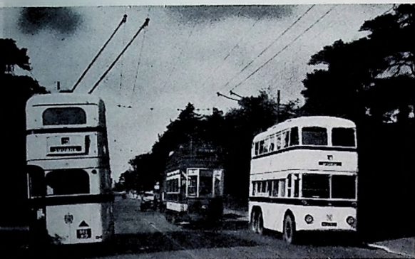
Trolleybuses were used in many places as tram replacements. Here, two Bournemouth M52s are seen with one of the trams they replaced
