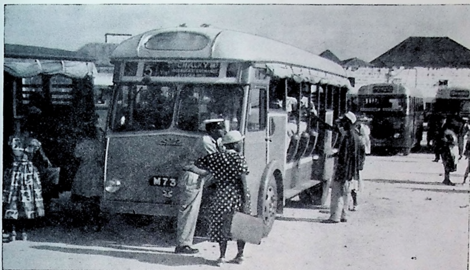
IN BARBADOS, toast-rack buses are popular. In heavy rain the canvas side covers can be let down. This Albion Claymore is operated by the Boston Bus Co. (Block by courtesy of "Leyland Journal").
