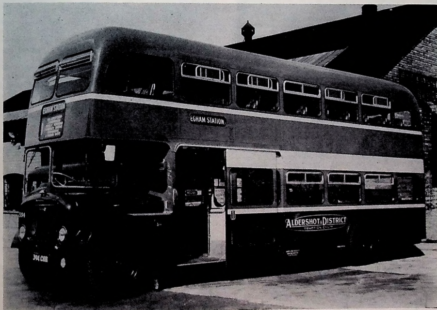
A letter on page 215 mentions Aldershot & District's Mark I Dennis Loline, which have 68-seat rear-entrance East Lancs bodywork. The company is now taking delivery of an order for 57 Loline 111s with 68-seat forward-entrance bodies by Alexander. By the beginning of last month, ten had been completed but only one (394) was in service. Since it came at the end of July, 394 has been used on services 1, 2, 3c and 4 (Aldershot/Camberley/Egham and Camberley/Old Dean estate). (Block by courtesy of Aldershot & District Traction Co. Ltd.)
